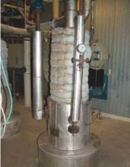
The pressure tank of the Presco system runs through a floor. Here pressure is elevated to 25 bar and temperatures rise to 300°C. At the bottom the exhaust pipe runs into the expansion tank.
