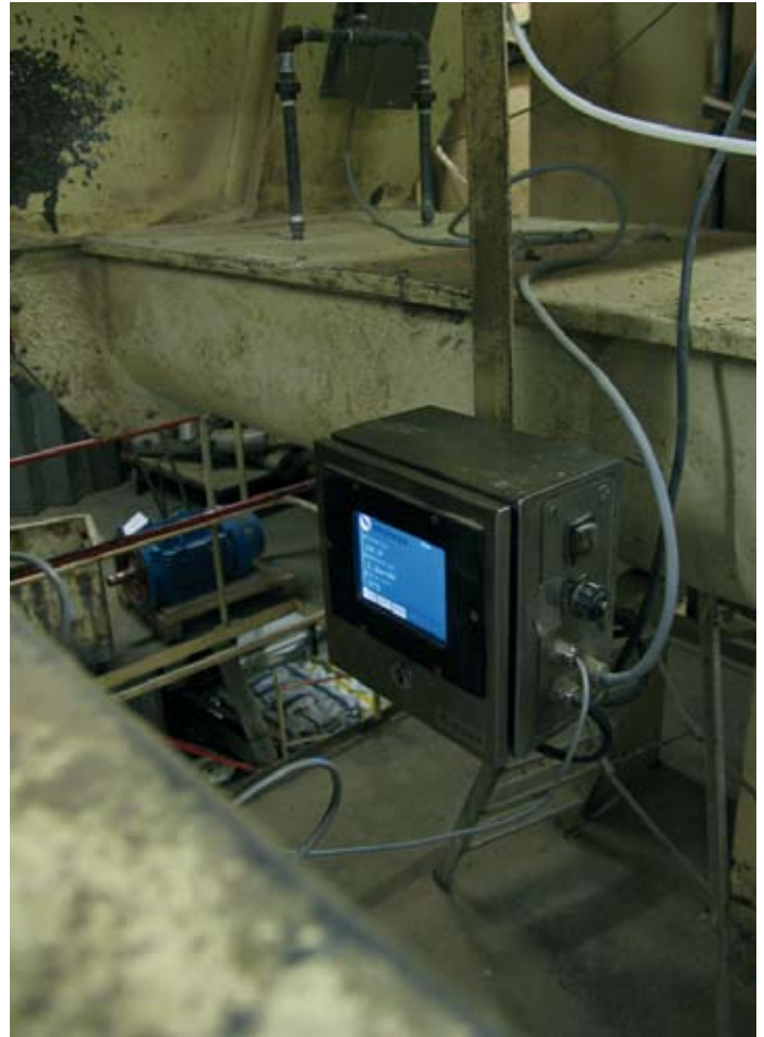
Moisture metering installed in a conveyor.
