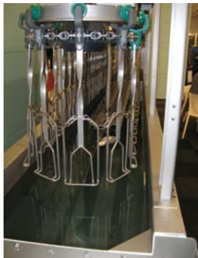
Thanks to a new technique of water pressure, scalding takes only three minutes, rather than 3.45 minutes previously, thus causing considerable energy saving.
