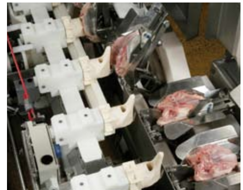
The new Stork semi-automatic loading module, places breast caps accurately onto a V-shaped holder.
