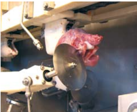
Based on very precise measuring, the Linco 656 fully automated deboner accurately adjusts for critical cutting of the shoulder and wishbone areas.
