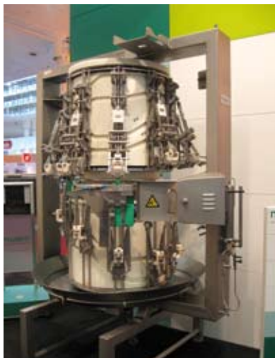
Tenderloins remain attached to the carcass with the Meyn HQ breast deboner. Onwards the machine pulls off the tenderloins from the tendon.
