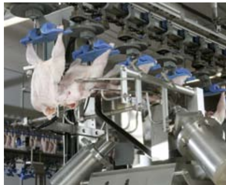
Stork developed an in-line "Wingstick" module. In this machine, the first wing joint is rolled up the bone and marinated on wards.
