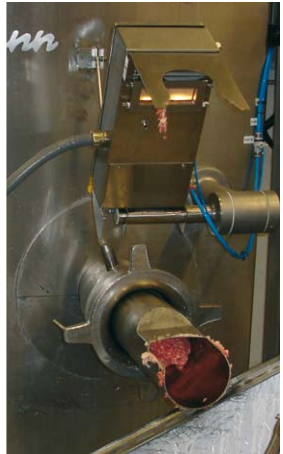
The NIR sensor above the grinder outlet in idle position.
